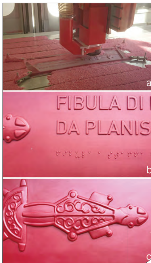
Fig. 12. Cornici e pannelli tattili in Corian DUPONT. Corian DUPONT tactile frameworks and panels.
