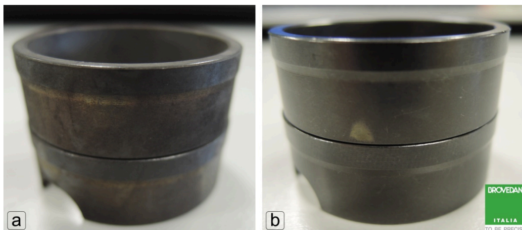
Fig. 6.38 Workpieces status after heat treatment (a) and after current polishing strategy (b)
