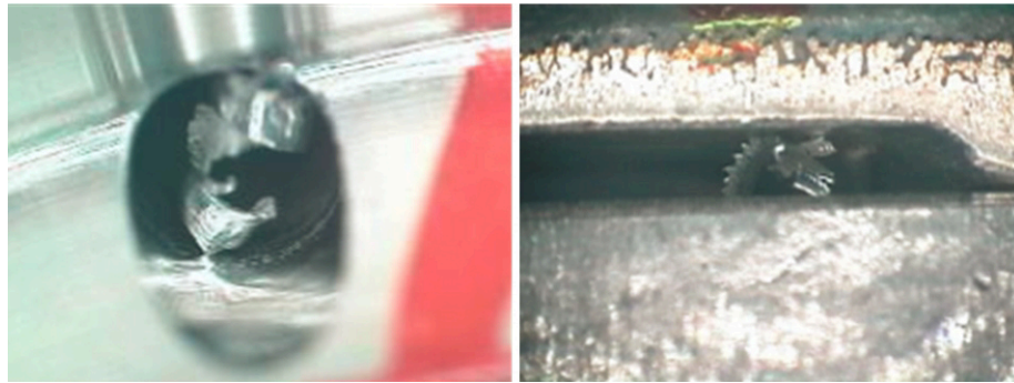
Fig. 7.7 Rough or semi-finishing machining contaminants, which in general are cutting oil and metal or plastic chips: they can obstruct holes or can remain in cavities (Courtesy of Brovedani SpA)
