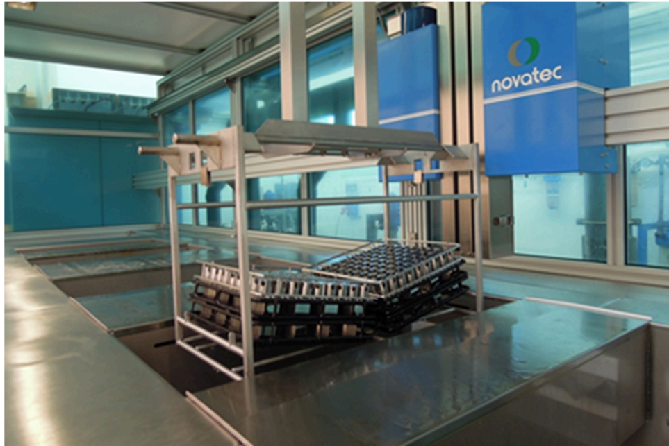
Fig. 7.3 Particular of multi-tank washing machine based on U.S. technique (Courtesy of Brovedani SpA)
