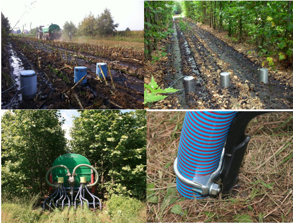
Fig. 4: Chambers methodology for the comparison between Maize and Platanus Hispanica and trailing hose technique applied in Tezze sul Brenta
