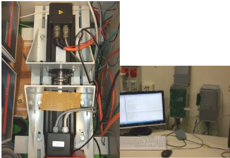
Fig. A.1. Experimental setup for the SM-PMSM for the back-EMF and LF-injection based sensorless control (3.5, 3.6.2, 3.7.3 and 4.4.3).
