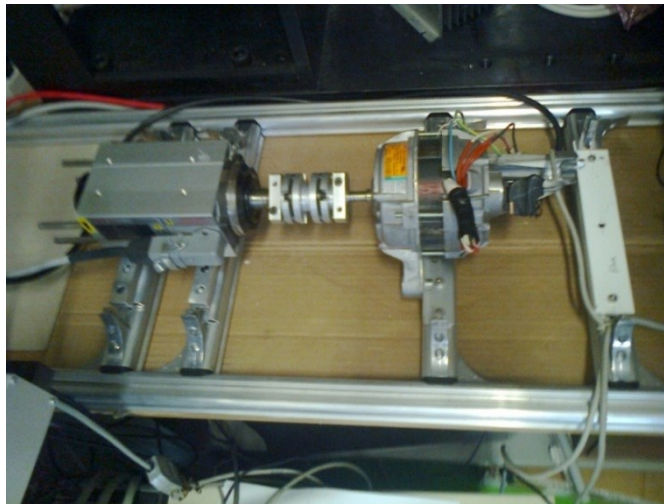
Fig. A.3. Experimental set-up for the the flux-weakening control and PWM excitation sensorless (5.4.7 and 4.3.5).
