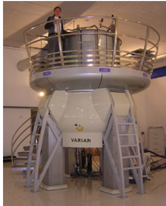
(a) A 21 T/900 MHz NMR spectroscope.
