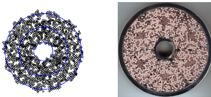
Figure 4.10: View of EUTF3-EAS sample model discretization and cross-section of a TF CICC (courtesy of ITER organization).
