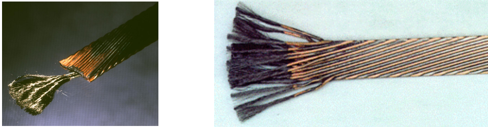
Figure 2.11: LHC Rutherford cable (© CERN). In both images, the copper matrix of some strands is etched, showing the Nb-Ti filaments.
