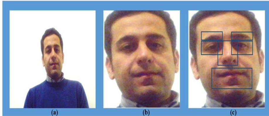
Fig 2-10 Face detection steps: (a) full frame photo (b) Zoom on face (c) feature candidate areas
