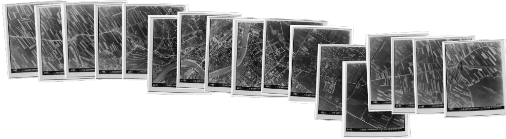
Figure 5.7: an example of a sequence of exposures taken by the Royal Air Force (RAF) during WWII (from the AFN archive). The photos are placed in their relative positions by panoramic stitching, using [13]. MiBAC-ICCD, Aerofototeca Nazionale, fondo RAF ©.
