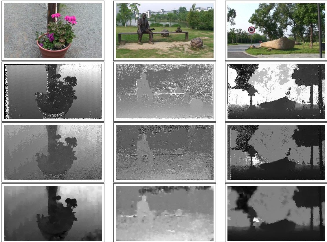
Figure 5.4: from top to bottom: the reference frame, the qualitative Best Map (manually selected), the result of Kalman-T (temporal-only) and the result of Kalman-ST . Images are automatically scaled in the range [0,255] , hence the gray levels change from row to row. Full resolution images can be seen at [77].
