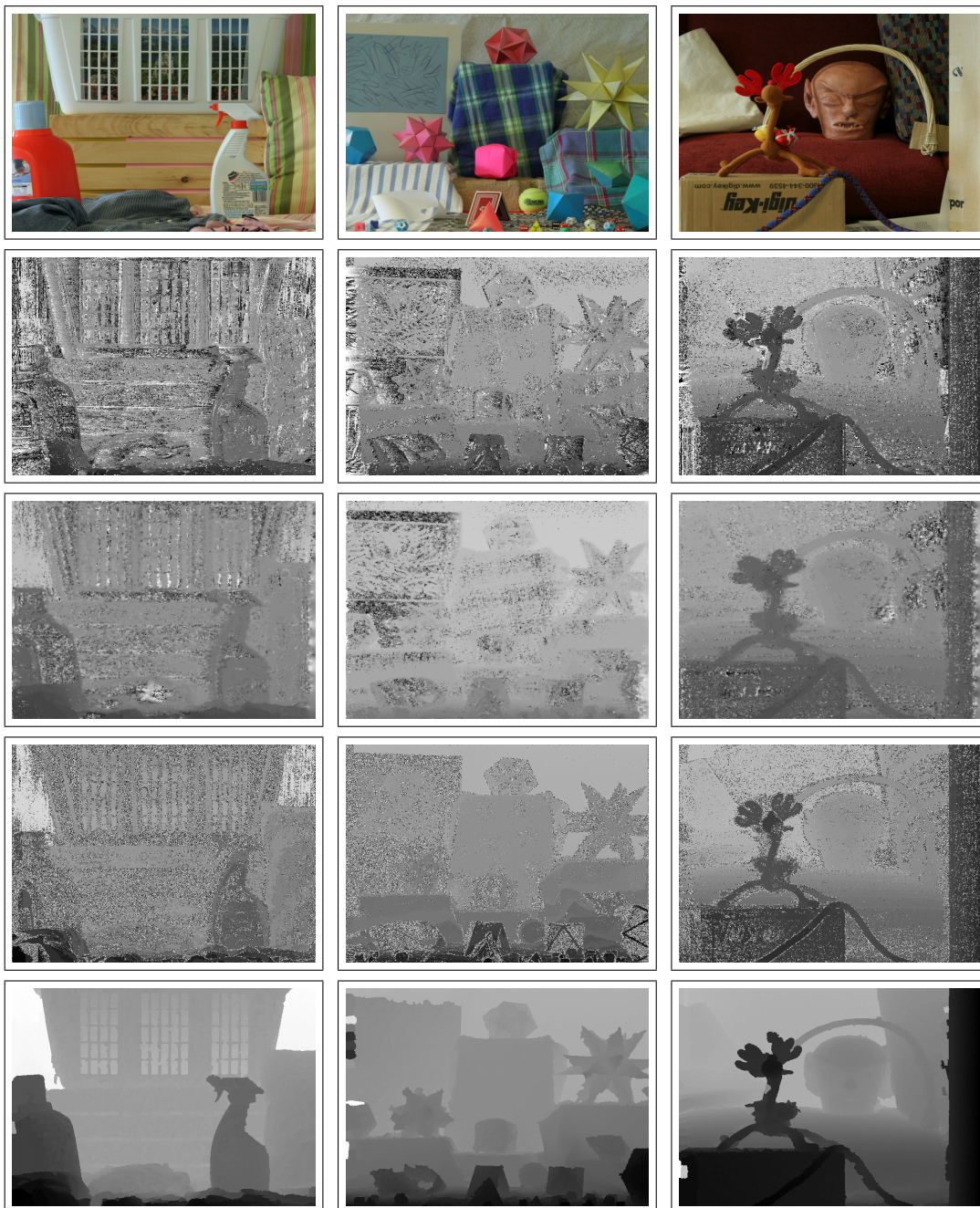
Figure 5.2: From top to bottom: the reference frame, the Best Map , the result of MKS , the result of Kalman T (temporal-only) and the result of Kalman ST . Images are automatically scaled in the range [0,255] , hence the gray levels change from row to row. Full resolution images can be seen on line [77].
