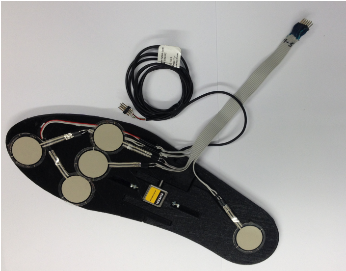
Fig. 3.8 – The whole insole with the five FSRs and the load cell.
