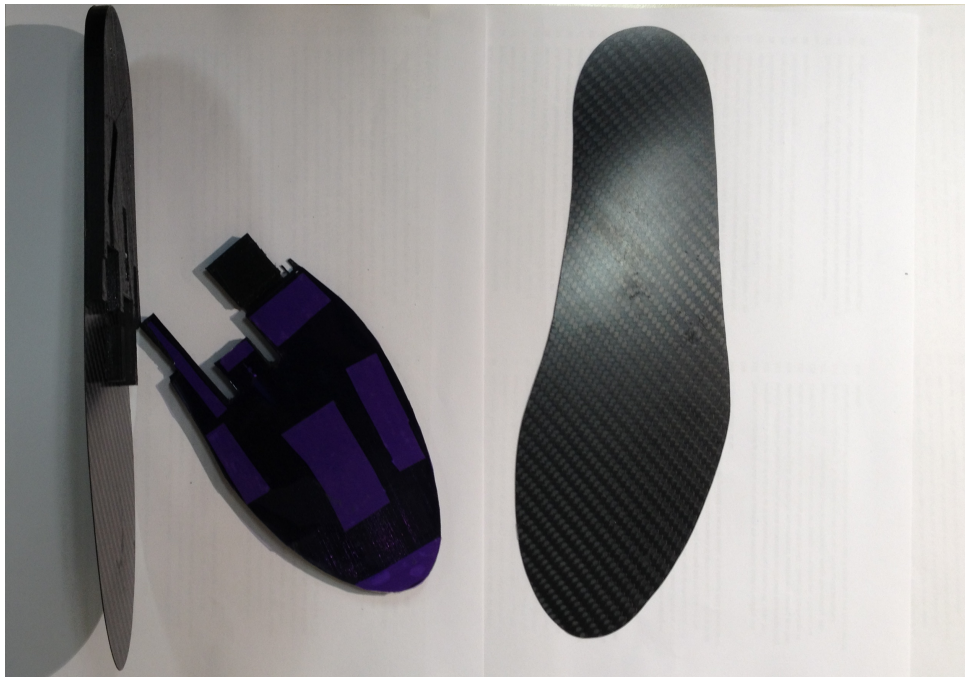
Fig 3.4 - The two TPU semi-sole with the kapton polyimide film
