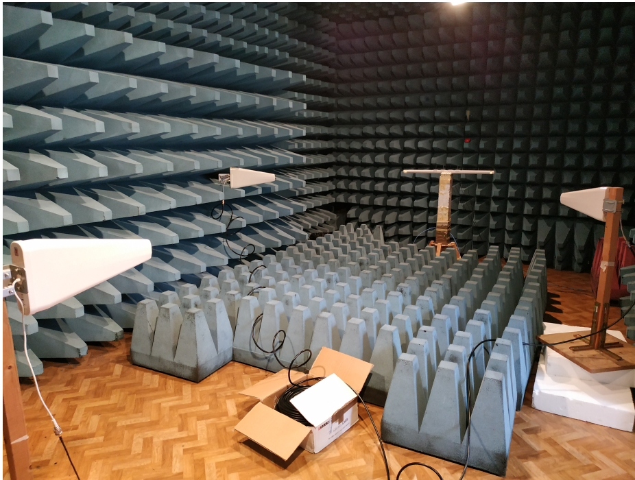
Fig. 6.9 Picture representing the set up of the second scenario in the Anechoic chamber
