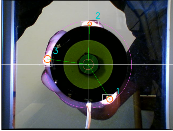
Figure 5.2: Finger-tracking: a Python application detects the position of three illuminated fingertips (small red circles) bounded within a circular region (large red circle enclosing the cylinder). The thin white cross marks the center reference.
