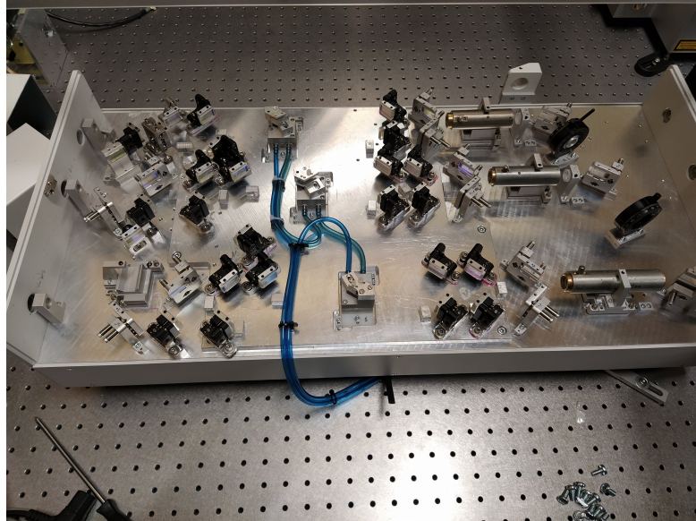
Figure 4.16: The picture shows the amplifier for the 1.26 \mu\text{m} laser beam. The black and some of the grey mounts supports for the mirrors needed for all the passes. In the center of the image, the three Cr:forsterite crystals inside their heat sink holders. The beams from the 1.06 \mu\text{m} pump arrives from the right.
