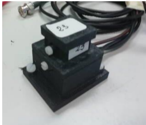
Figure 3.8: A \text{LaBr}_3(\text{Ce}) detector read by SiPM. The 3D printed cases of these detectors are designed to be disassembled for a fast check.
