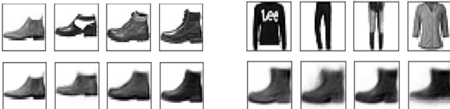
Figure 3.8: Top row: normal (left) and anomalous (right) samples from the Fashion MNIST test set. Bottom row: the reconstructed images.
