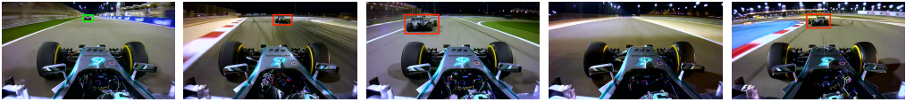
Figure 1.1: Example of a visual object tracking problem. The images are sampled from the frames that compose the video acquired from the camera mounted on a Formula 1 car. The target object to be tracked by an algorithm is the other Formula 1 car in front of the chasing one. The algorithm is first given the target state (represented in green in the leftmost image). Then, it should be able to recognize the object of interest and provide its localization by proposing its successive states (represented by the red rectangles) for all the frames. The object could also disappear from the scene captured in the video and hence not being present in some frames.
