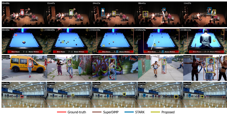
Figure 4.4: Qualitative examples of the tracking ability achieved by the proposed algorithm in comparison with the baseline trackers STARK and SuperDiMP. The first column of images presents the first frame of each video. In the top-left corner of each frame the time elapsed since the beginning of the video is reported. Overall, our solution permits to fuse the capabilities of the underlying trackers and consequently achieve a more robust target tracking along the videos.
