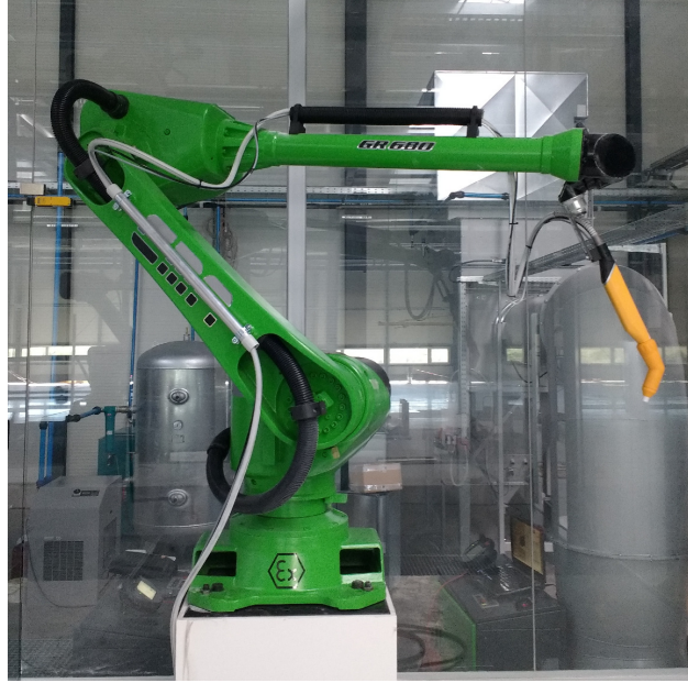
Figure 1.8: An industrial spray painting robot.
