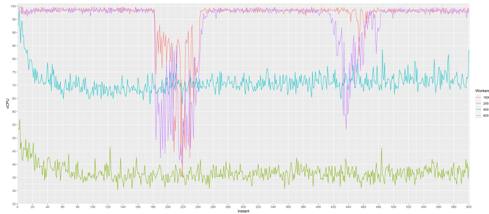
Figure A.23: CPU usage of the dedicated server solution during each round of the test.
