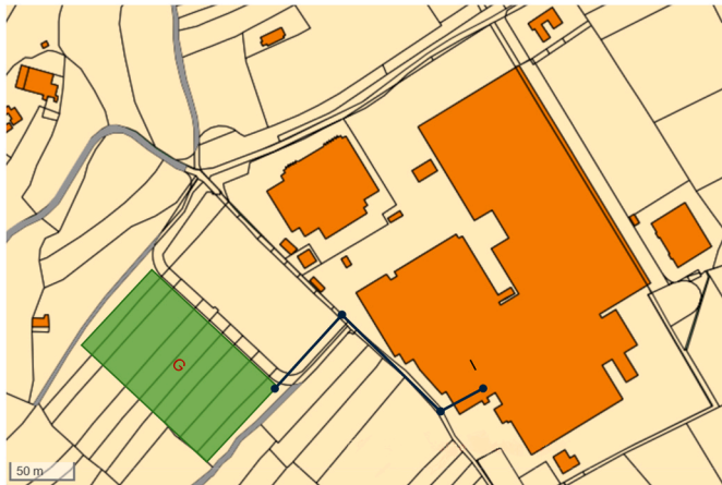
Fig. 5. Layout of the buildings and proposed DH network branches – Case study 2.
