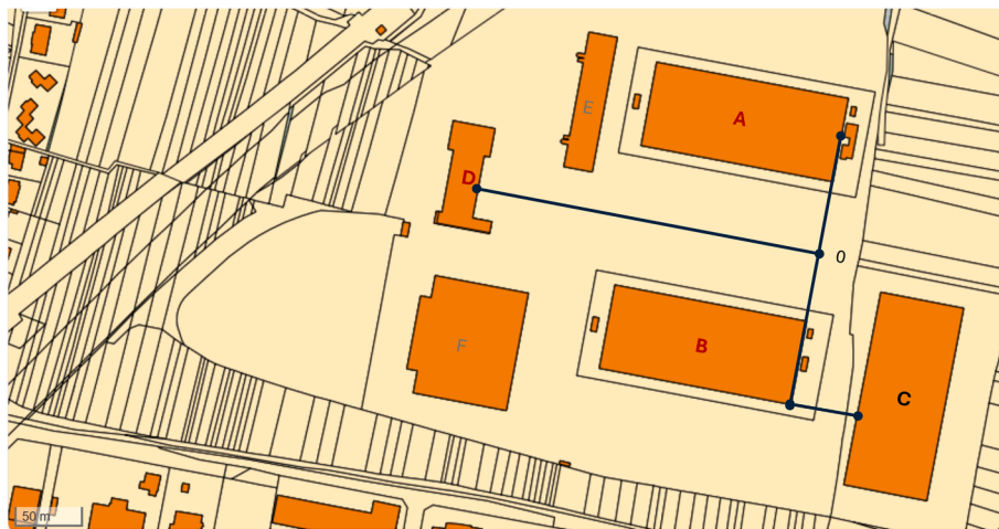
Fig. 3. Layout of the buildings and proposed DH network branches – Case study 1.
