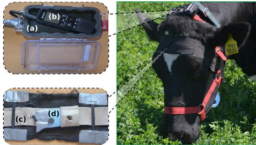
Figure 6. Recording system used to measure acoustic signals (Martinez-Rau et al., 2023).
