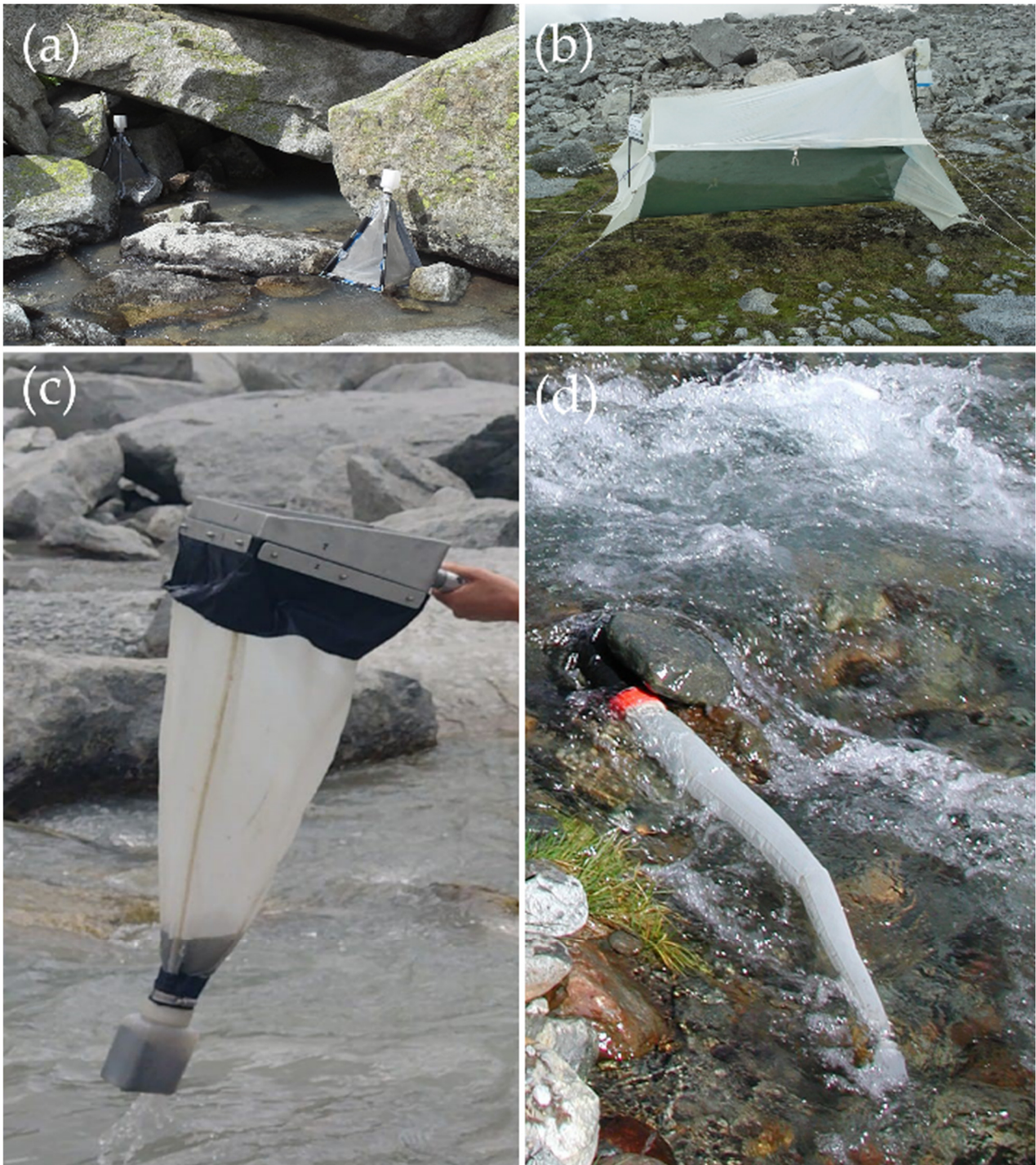
Figure 2. The four sampling methods used: (a) emergence trap; (b) Malaise trap; (c) pond net; (d) drift net.
