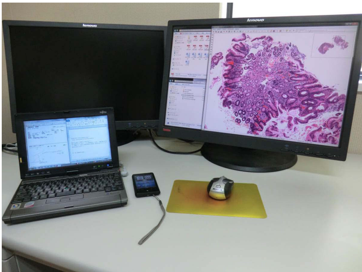
Figure 2(abstract S4) Actual working desk of remote diagnosis Notebook PC was connected to the web through mobile telephone network. Another display is also connected to the notebook PC, and diagnosis was done under dual display condition.
