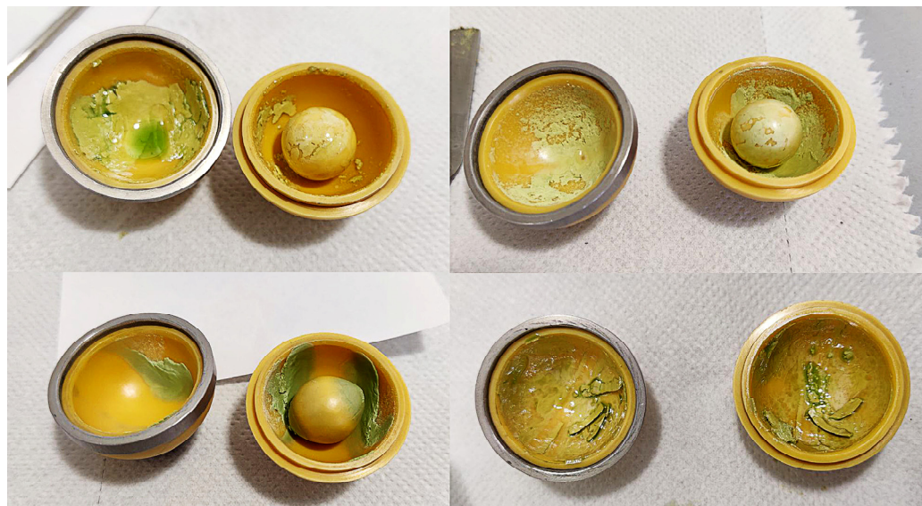
Figure 3. Pictures of Ni/CeO 2 samples milled with H 2 O-rich precursor salts. The same synthesis of Ni/CeO 2 was carried out using Ni(NO 3 ) 2 ·6H 2 O, a heavily hygroscopic salt, and ceria powders; the preparation was repeated with the same procedure on different days characterized by different levels of relative atmospheric humidity. The results varied on a daily basis as different levels of humidity were present; during the most humid days, the amount of H 2 O adsorbed by the salt was enough to create a wet layer and separate the finely dispersed Ni nitrate salts from the ceria.
