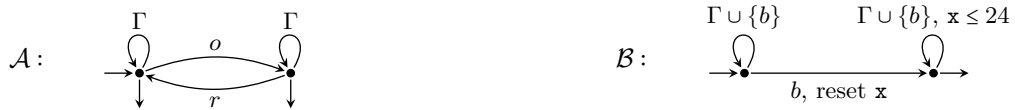
■ Figure 1 Left: a finite automaton \mathcal{A} recognising \Gamma^*(o\Gamma^*r\Gamma^*)^* . Both states of \mathcal{A} are accepting, but invalid streams do not admit any run. Right: a timed automaton \mathcal{B} with single clock x .
