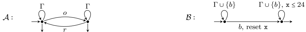
■ Figure 1 Left: a finite automaton \mathcal{A} recognising \Gamma^*(o\Gamma^*r\Gamma^*)^* . Both states of \mathcal{A} are accepting, but invalid streams do not admit any run. Right: a timed automaton \mathcal{B} with single clock x .
