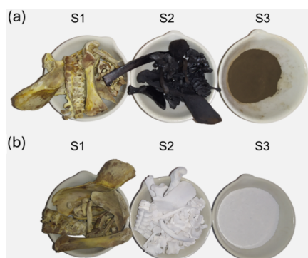
Figure 1. Steps of the biogenic nanohydroxyapatite synthesis. S1) Raw material; S2) calcinated material before the ball milling; S3) calcinated material after the ball milling, at (a) 300 °C and (b) 700 °C.
