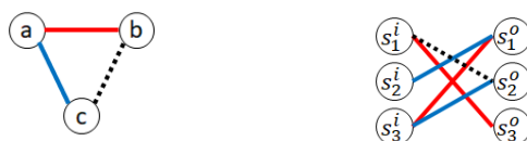
■ Figure 2 An example of the difference between connection caching versus caching in matchings. (left) With k = 2 max degree and n = 3 nodes, all the connections can be cached simultaneously, but not in 2 matchings, red and blue. (right) Bipartite example: Caching the edge (s_1^i, s_2^o) (i/o for in/out) is not possible without changing the matchings (red: \{(s_1^i, s_3^o), (s_3^i, s_1^o)\} ; blue: \{(s_3^i, s_2^o), (s_2^i, s_1^o)\} ), although both s_1^i and s_2^o only have a single connection.
