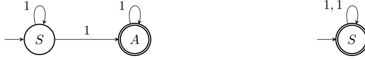
■ Figure 1 NFAs computing the functions 1^n \mapsto n and 1^n \mapsto 2^n respectively. Edges with a multiplicity of 2 are denoted by listing the edge label twice.
