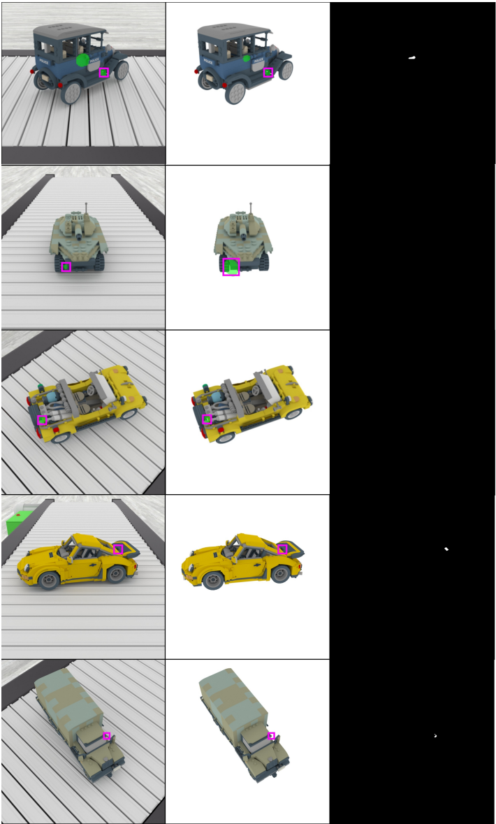
Figure 6.5: Qualitative comparison of detection errors. Examples of false positives and false negatives are highlighted with boxes. First column: proposed method; second column: SplatPose+; third column: ground-truth masks.
