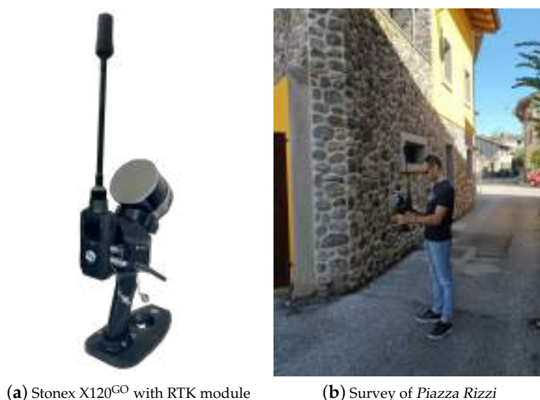
Figure 3. (a) The SLAM device (Stonex X120 GO [39]) used for reference data acquisition and (b) the operator during the survey of the first case study ( Piazza Rizzi ).
