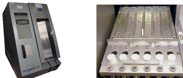
Figure 4.4 BioRobot® EZ1 system workstation (Qiagen N.V., Germany) and preparation of DNA extraction using EZ1 DNA Blood 200 \mu L Kit (48).
