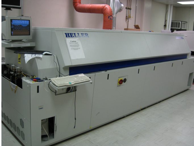
Figure 7.1: Reflow oven typically used in the semiconductor industry (photograph by Nelatan, distributed under a CC BY-SA 3.0 license).
