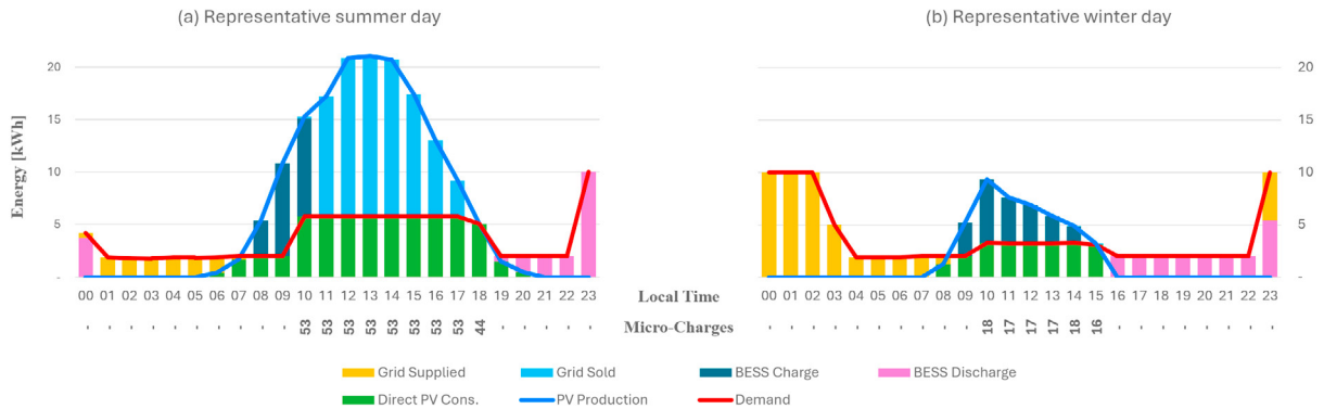
Fig. 5. Energy flows with microcharging strategy for a Tuesday in June (a) and December (b). Numbers below each graph indicate total robots scheduled for microcharging during each hour.
