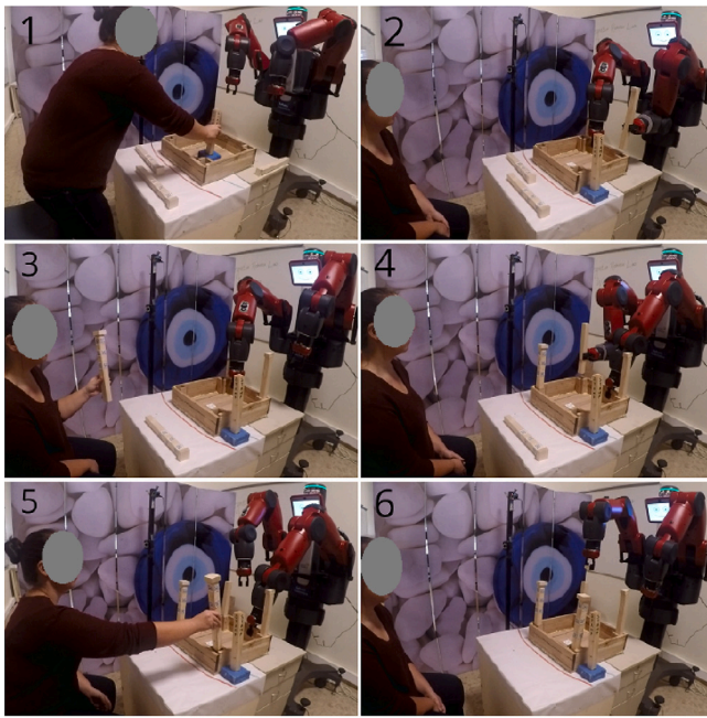
Fig. 6. Human–robot collaboration for the assembly of a table with a Baxter robot [49].
