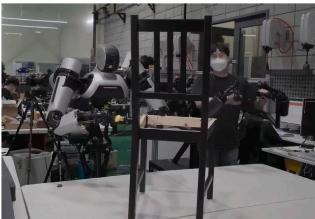
Fig. 9. An operator guides the robot to perform the assembly of a chair [54].
