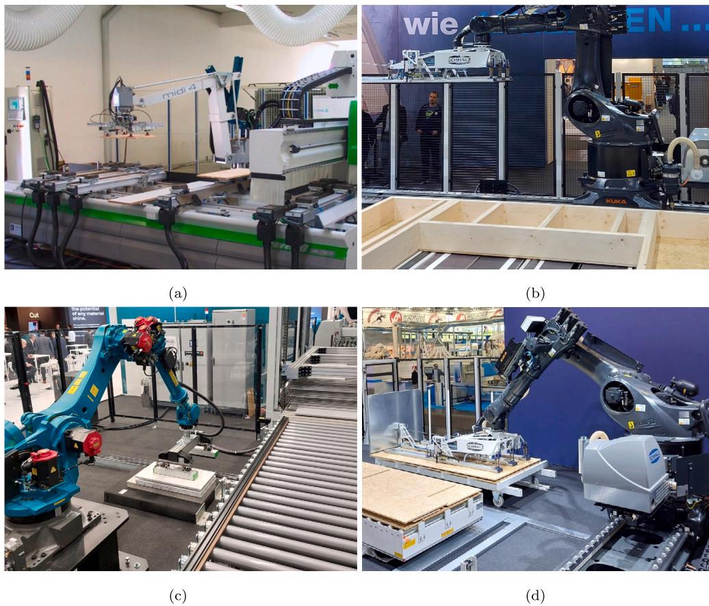
Fig. 1. Examples of pick-and-place of large and heavy components for loading a wood processing center [10] (a), and for moving wooden panels from the storage to the conveyor (b), (c), (d).
