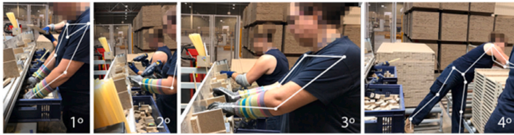
Fig. 10. Manual assembly and skeleton tracking for evaluating the ergonomic conditions of workers [59].
