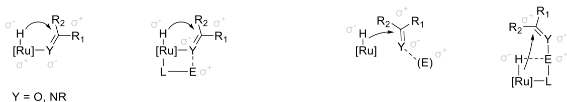
Figure 39 – The TH reaction has different possible reaction mechanisms, and here, four examples of the key reaction steps involving the hydride transfer have been reported. From left to right, 1) inner sphere, 2) inner sphere ligand assisted, 2) outer sphere, 3) outer sphere ligand assisted.
