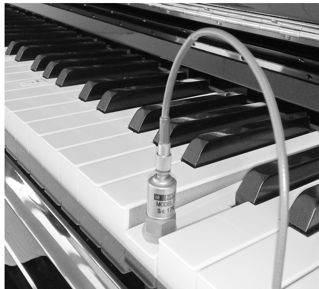
Figure 9. Piano keyboard vibration recording setup. A measurement accelerometer is attached with adhesive tape to a key that is being played remotely via MIDI control.
