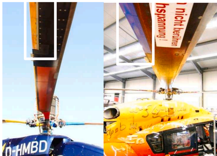
Fig. 31. Active rotor ADASYS vs Blue Pulse (From Ref. [309]).
