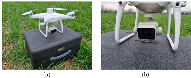
Fig. 4. (a) The DJI P4 multispectral UAV; (b) the multispectral and RGB cameras.
