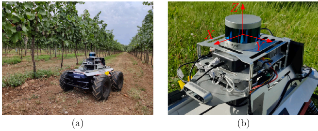
Fig. 5. (a) The Scout 2.0 mobile robot; (b) close view of the robot electronics and LiDAR sensor.
