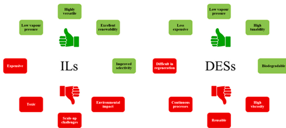
Fig. 10. ILs and DESs pros and cons in hydrometallurgical recycling from spent LIBs.
