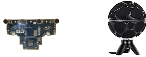
Figure 5. a) Sony PlayStation Eye (PS3 Eye) where the 4-microphone linear array is visible on top of the device and b) Zylla ZM-1 consisting of 19 microphones organized in a spherical array
