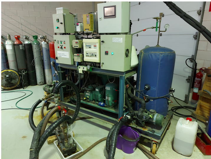
FIGURE 3.4: Experimental water/propylene glycol mixture supply system
