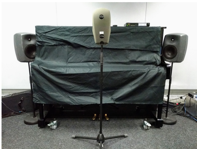
FIG. 3. (Color online) Recording setup with dummy head binaural microphone.
