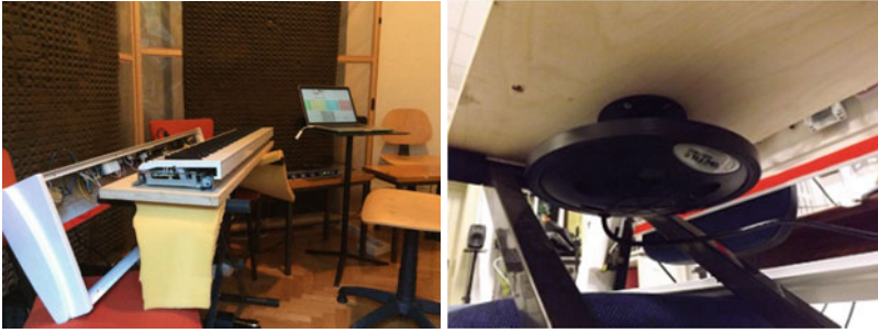
Fig. 12.12 Left: experimental setup. Right: transducer conveying vibrations to the keyboard
