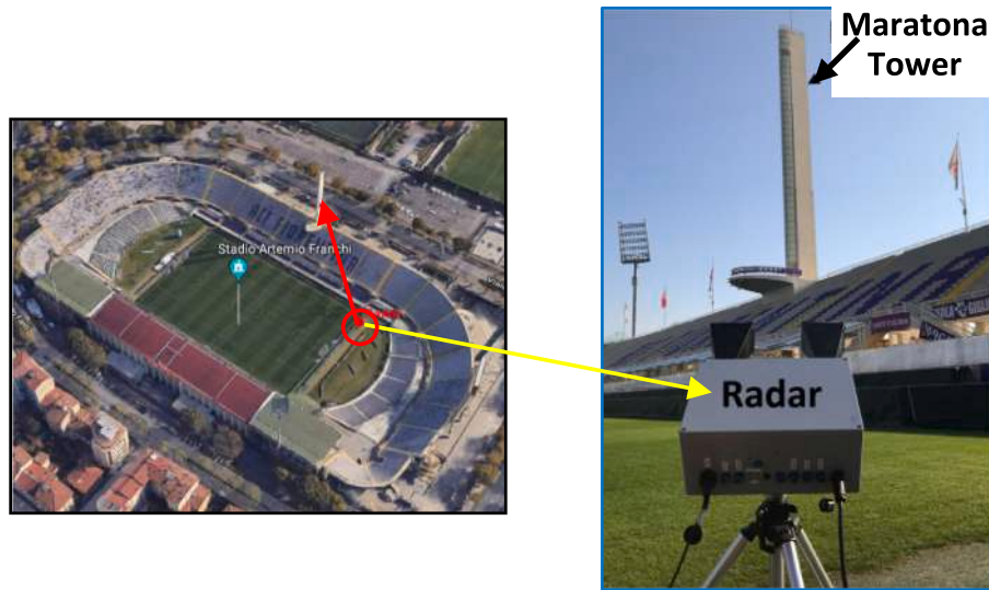
Fig. 11. Positioning of the radar sensor equipment within the playing field for a dynamic survey on Maratona Tower under wind action.
