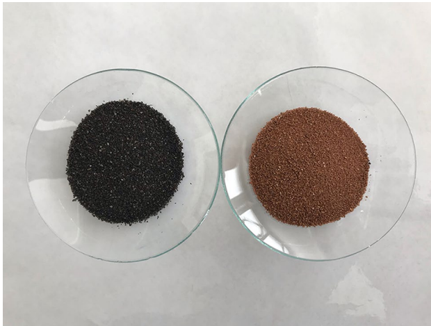
Fig. 3 Appearance of OS, before (left) and after (right) thermal treatment
