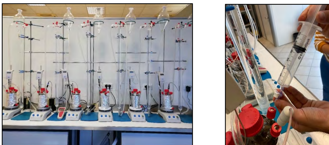
Figure 1. Overall view of the lab-scale system used for the AD experiment (left) and particular view of the biogas sampling from the headspace of one digester (right)
