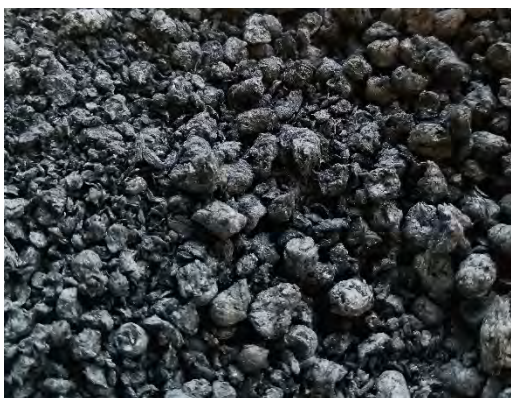
Figure 3: Char from slow pyrolysis of textile waste pellets.
