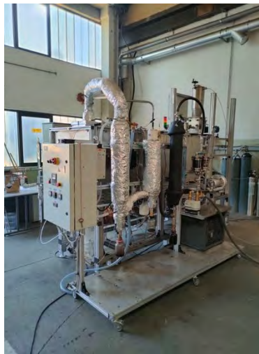
Figure 2: pilot scale pyrolysis unit integrated with the FCU.
