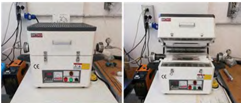
Figure 1. SAFTherm SANTE FURNACE experimental setup containing quartz tube
