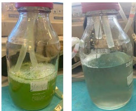
Figure 2. Appearance of the chlorella vulgaris microalgae solution before the beginning of the experiment (left) and after 5 h of treatment at 245 mA (right).
