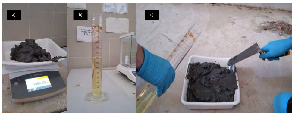
Figure 1. a) 1.5 kg of sediments; b) 150 ml of diesel oil; c) Mixing.
