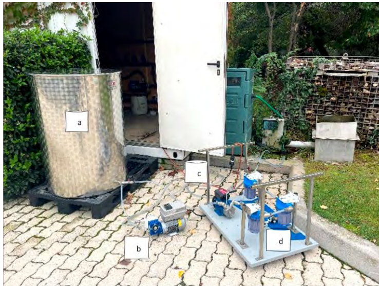
Figure 1 - System for wastewater collection and filtration. 1) 400 L stainless steel tank for effluent 24 h accumulation, b) peristaltic pump for tank loading, c) centrifuge pump for rapid filtration, d) stainless-steel filter cartridges (300-10-2 \mu\text{m} ) for solids capturing.
