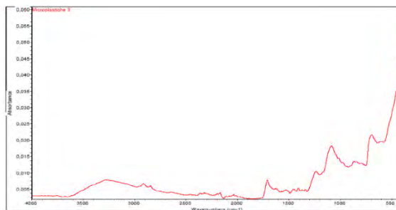
Figure 2. FTIR emission spectrum after Fenton treatment.
