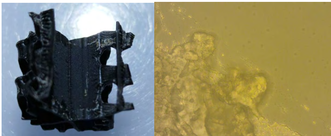
Figure 3 The carrier's internal surface shows an incipient biofilm after 38 days (sx). Detail of the biofilm (40 x magnification).
