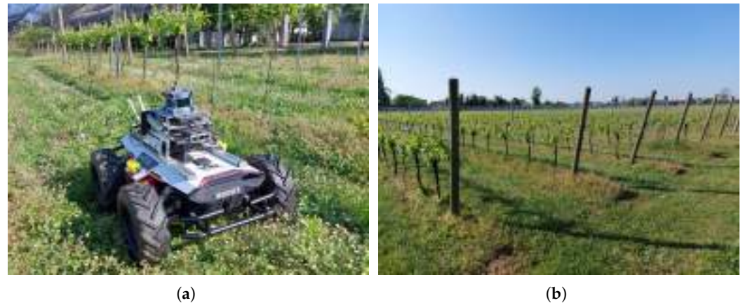
Figure 4. Scout 2.0 mobile robot used in the experimental tests (a); vineyard of the A. Servadei farm of University of Udine, Italy (b).
