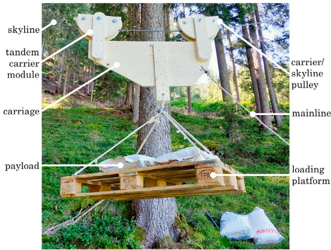
Fig. 8. Skyline tensile force observer test setup consisting of a wooden carriage with a loading platform suspended by a skyline.
