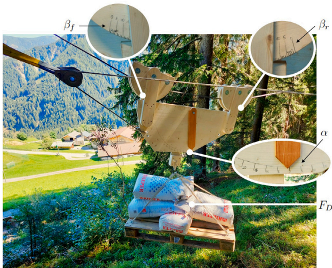
Fig. 11. Relative rotation of the carrier modules and carriage inclination read from the carriage.
