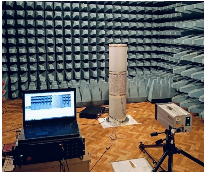
Figure 25: laser vibrometer measurement setup
