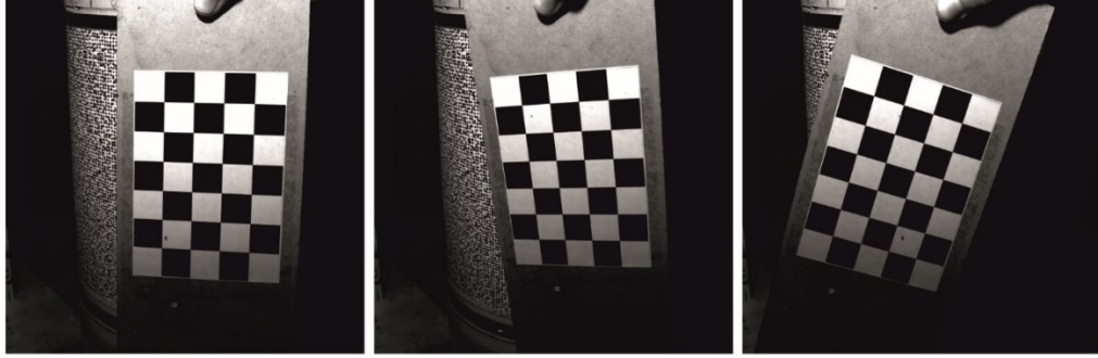
Figure 16: three different views of a chessboard used for camera calibration
