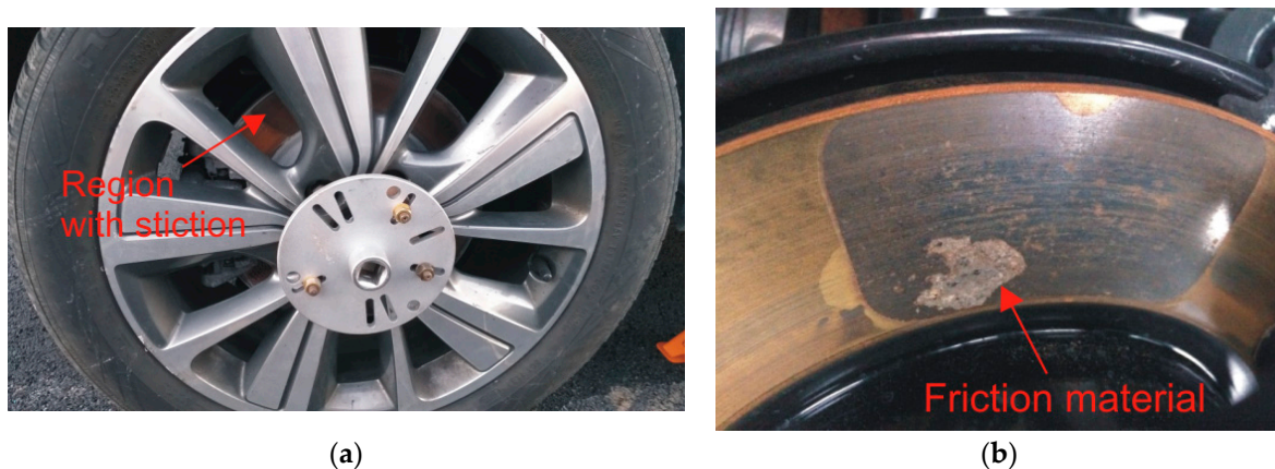
Figure 2. Example of corrosion stiction in an automotive braking system: (a) region of the brake disc showing stiction; (b) adhesion of friction material on the brake disc. Courtesy of ITT Italia S.r.l. (Barge (CN), Italy).
