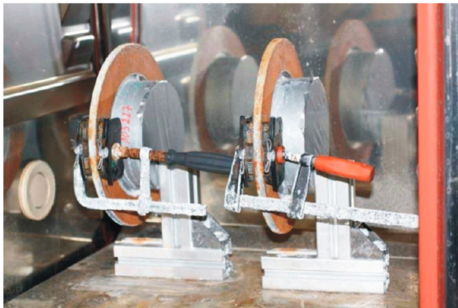
Figure 5. Example of exposure of a brake pad–disc couple in a humidity chamber. Courtesy of ITT Italia S.r.l. Barge (CN), Italy).
