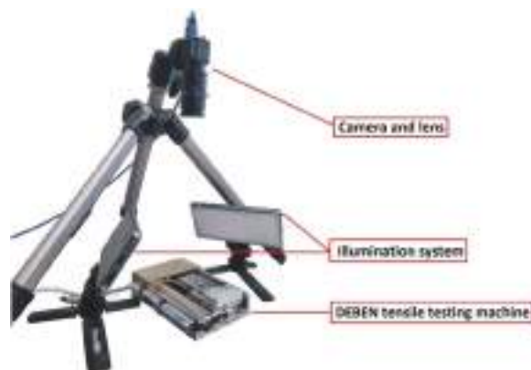
Fig. 2.4. Complete testing setup consisting of a tensile testing machine, camera, lens and LED lights.
