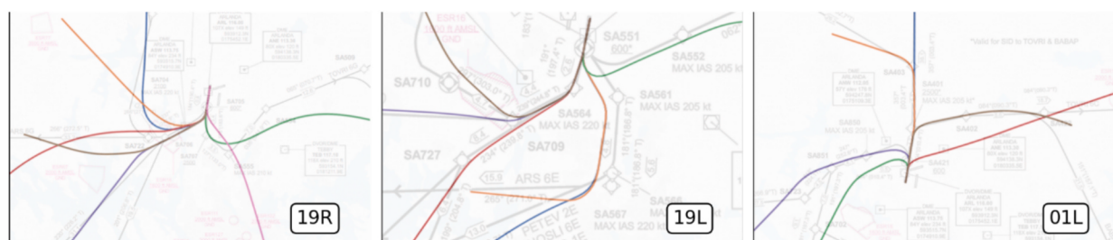
Fig. 4. Comparison between 2026 SIDs (grey lines in the background) and centroids of departure clusters based on 2022 flight tracking data (coloured lines) for three runways at Arlanda Airport.
