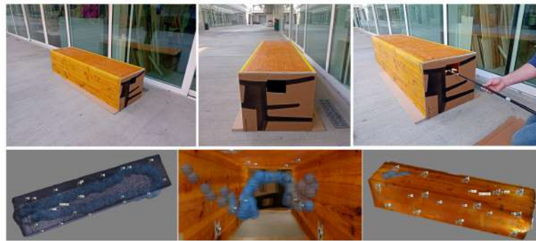
Figure 4. The rectangular box used in the first test ( top row ) and the visual results of the photogrammetric processing ( bottom row ).
