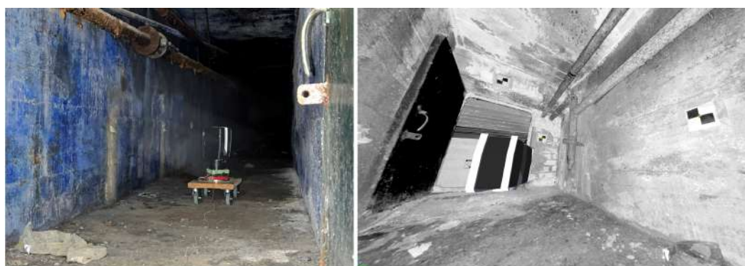
Figure 5. The laser scanning acquisition of the tunnel used in the second lab experiments.
