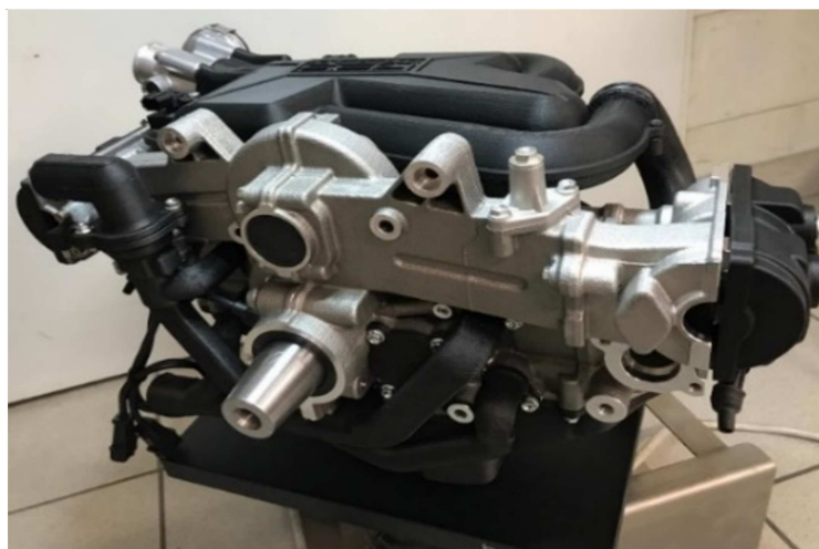
Figure 9.3: Prototype of the internal combustion engine.
