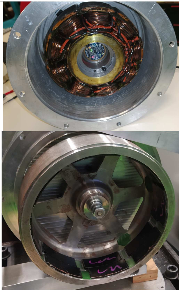
Figure 9.5: Prototype of the electric machine: stator (top) and rotor (bottom).
