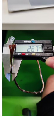
Figure 2.24: Wire diameter of 2.7 mm for a 130 \times 0.2 basic Litz wire configuration. The copper-to-wire-area ratio is 70 %, without considering the strand insulation. Hence, a slightly smaller number is expected
