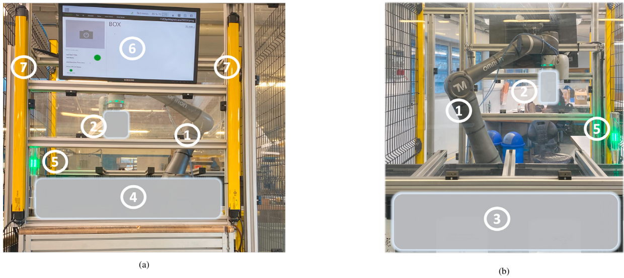
Fig. 2: Picture of the developed workstation: (a) front and (b) back. Some details are hidden on purpose to protect trade secrets.
